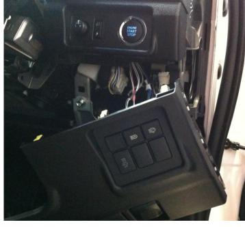
50. Due to CANBUS wiring system on vehicles fitted with LED headlights, there is no usable power supply/signal for the bullbar clearance lights on the connector at the head lamps.
